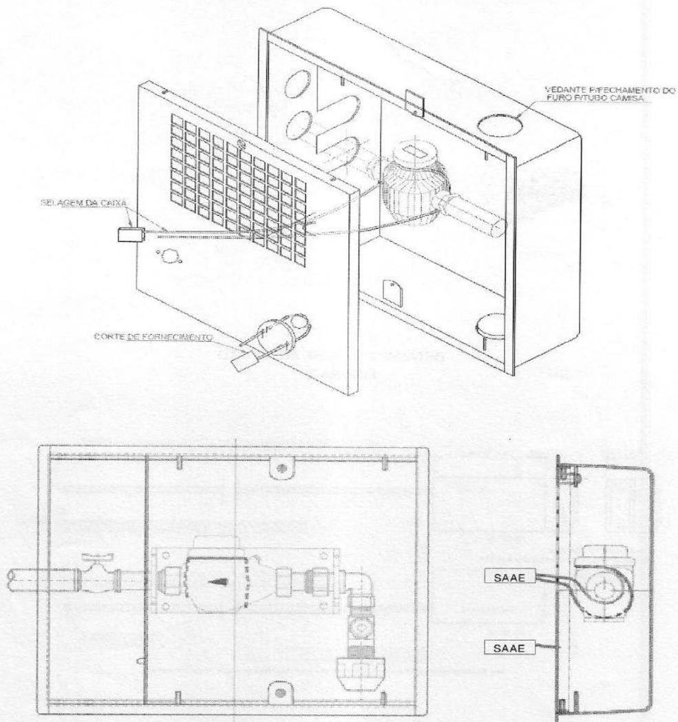
DETALHE DA INSTALAÇÃO DOS LACRES – DISPOSITIVO SIMPLES
